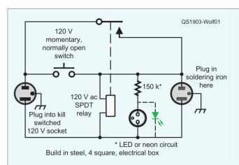
Figure 1 — The auto-kill soldering iron latching relay circuit is built into a 4-inch square electrical utility box. A bright pilot light serves as a reminder that the soldering iron is on. Once power is removed by the master kill switch, the circuit will remain off until the normally open activation switch is once again pushed.
